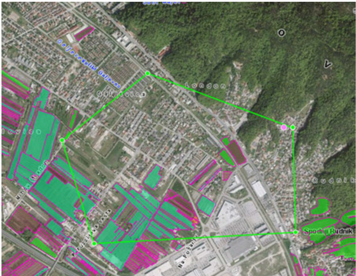
Figure 23: spatial tool for finding polygons which are included in the bigger drawn polygon.
