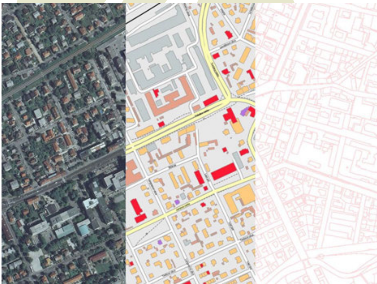
Figure 4: map view displaying three different kinds of data: on the left is orthophoto, in the middle raster spatial data and on the right vector spatial data.
