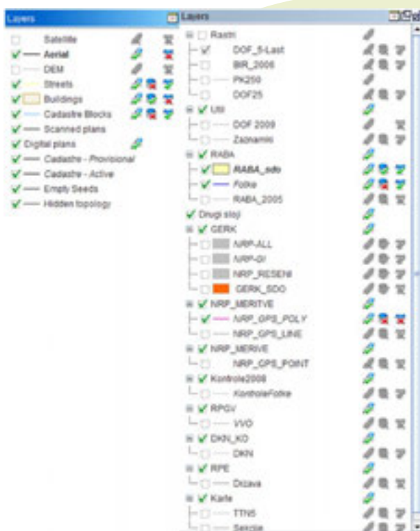
Figure 5: Layer control contents for two different applications: on the left is a cadastral application and on the right is a LPIS application with more layers
