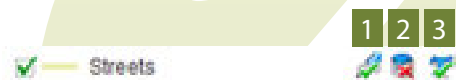
Figure 7: Layer control functions: if checkbox is checked, layer is turned on. Color shows how elements of the layer will be shown on map. If the name is bold, layer is selected for query. The first icon (1) shows enabling/disabling drawing of line boundaries, second icon (2) shows enabling/disabling shading of layer features and third icon (3) shows enabling/disabling of text annotation.
