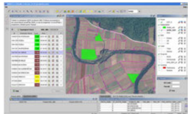
Figure 2: LPIS client application, displaying several selected land parcels, overlaid on orthophoto imagery. The panel on the left displays all parcels for a selected farmer.
