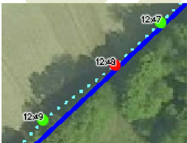
Figure 12: green GPS points were taken using EGNOS correction, red one without it, probably due to a shadow of the trees
